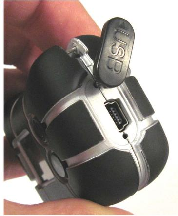
The camera is supplied by an integrated rechargeable Lithium-Polymer battery. Charging of the camera takes about 3 hours.
